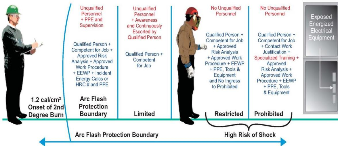
Example of Detailed Arc Flash and Shock Warning Label
